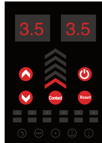
The pump lost connection or is running independently
