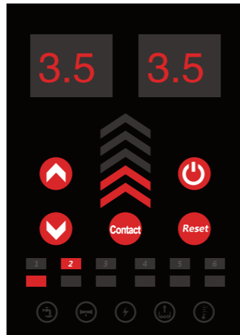
Pump 2 is the lead pump
