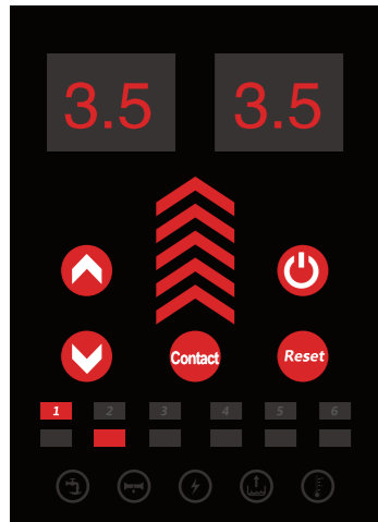
Pump 1 is the lead pump
